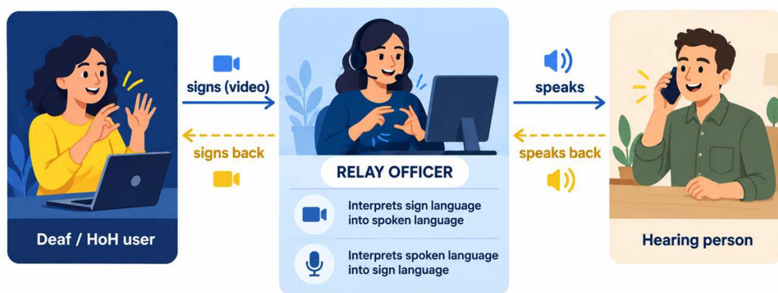
Figure 1. Video relay service: how a call is relayed between a deaf sign language user and a hearing person.
